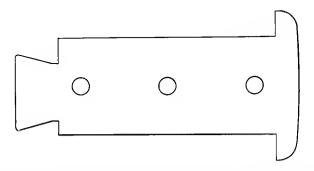
FIG. 72. Field core stamping of electrical steel for revolving armature alternator (Allis-Chalmers Co.) showing dove-tail tenon to be cast into frame.
